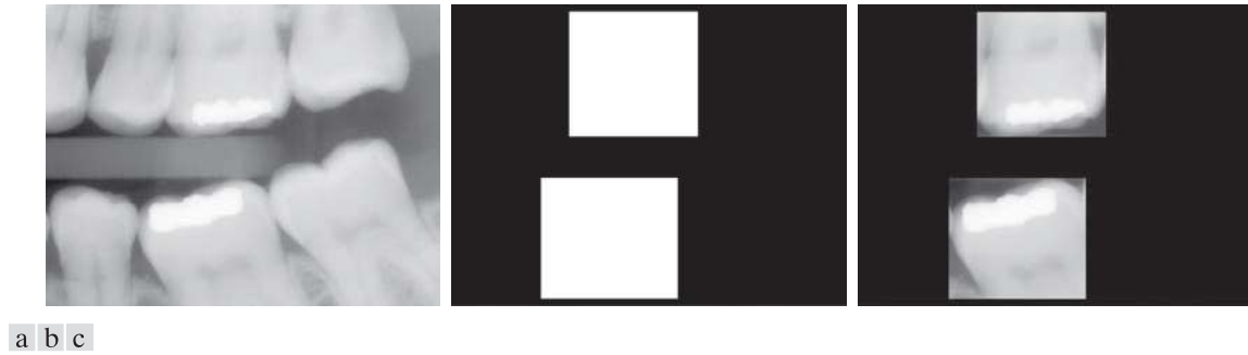
FIGURE 2.34 (a) Digital dental X-ray image. (b) ROI mask for isolating teeth with fillings (white corresponds to 1 and black corresponds to 0). (c) Product of (a) and (b).
