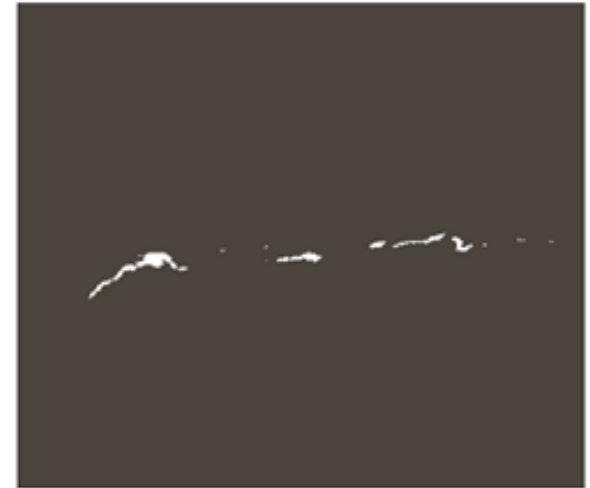
Seed image (99.9% of max value in the initial image). Crack pixels are missing.
