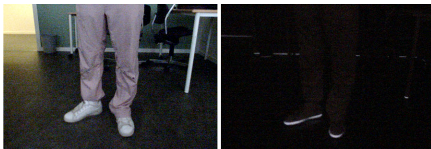
Fig. 12.4 Left: Image of a person's lower body. Right: Same image captured by a camera with a visual-light filter inserted and with infrared light sent out in a plane elevated a few centimeters above the floor
