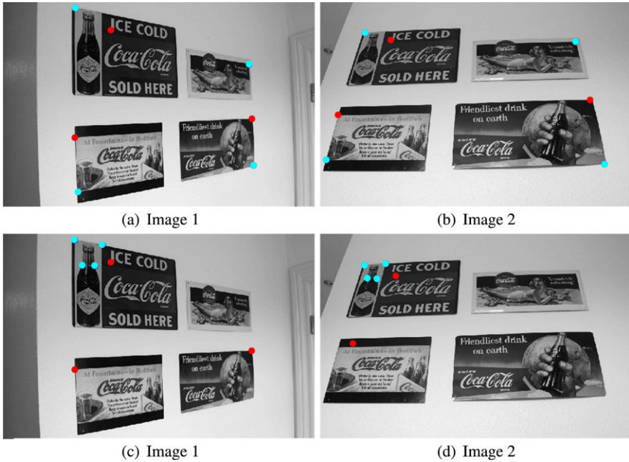
Fig. 10.7 The importance of choosing the four points far apart. The blue points are used for calculating the mapping between the two coordinate systems, whereas the red points are mapped from image 1 to image 2 using this mapping
