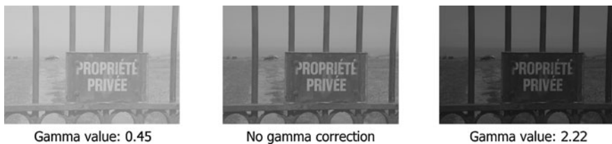
Fig. 4.6 Gamma mapping to the left with \gamma = 0.45 and to the right with \gamma = 2.22 . In the middle the original image
